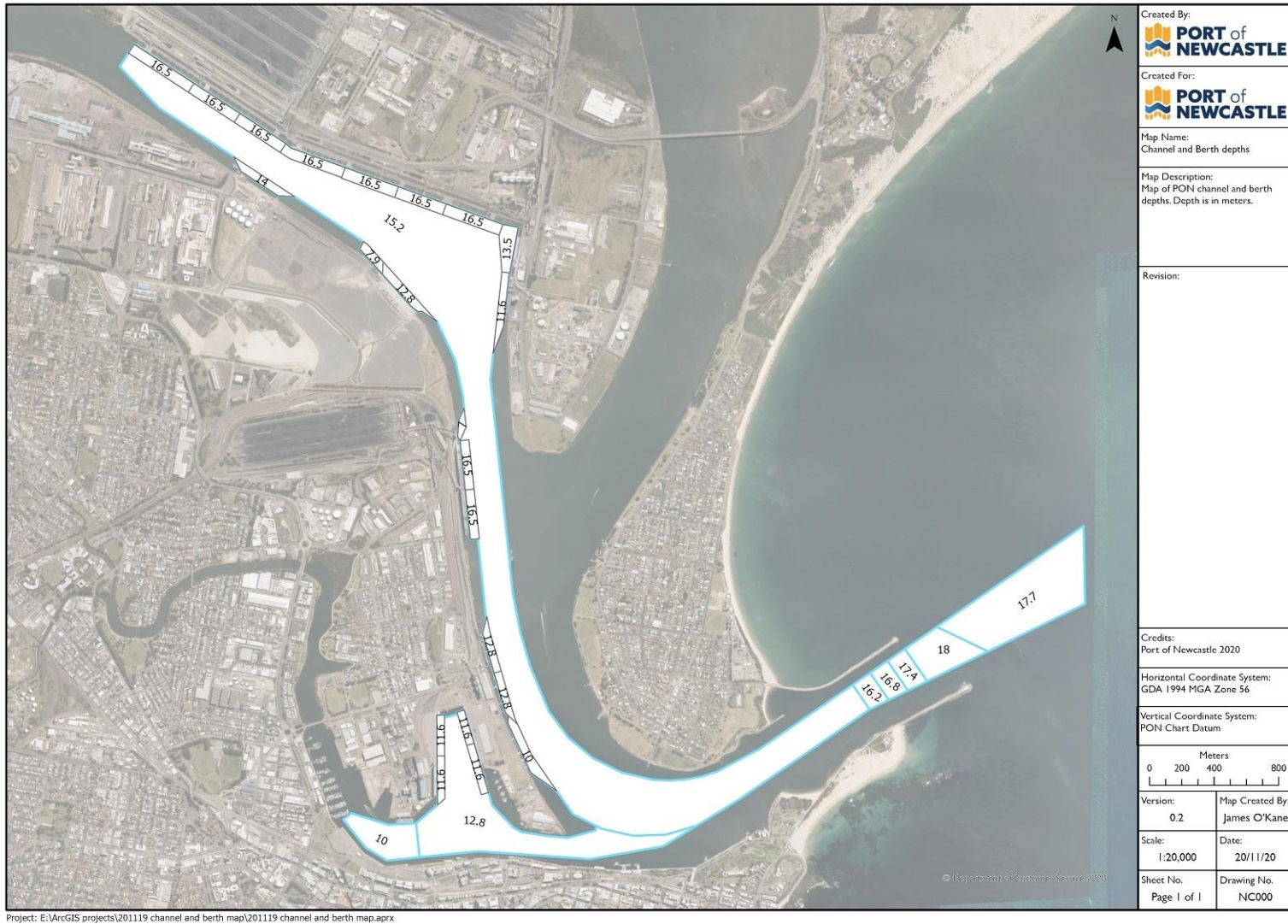
Figure 1 Declared depths within PON channels and berthing boxes
